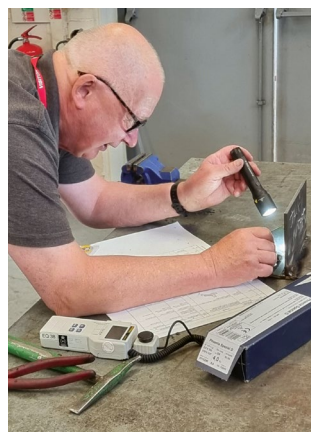
Figure 3: Keith Temperley (EngEPA assessor) reviewing a student's test piece for compliance with BS EN ISO 9606-1 Welder Qualification. Courtesy of EngEPA.
